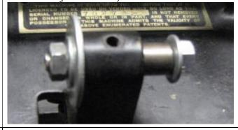
5. When done, the bearings should be visible like this. A couple drops of light oil through the top hole will be helpful.
